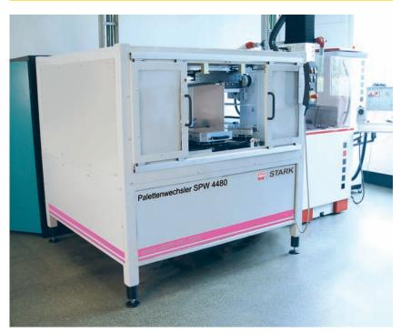
With its compact size, the SPW palette changer is easily installed in CNC machining centers. Depending on the equipment, up to 8 machine palettes can be loaded.
