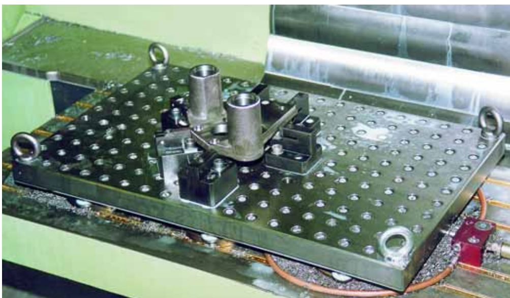
Perforated palette with deep drawing clamp
