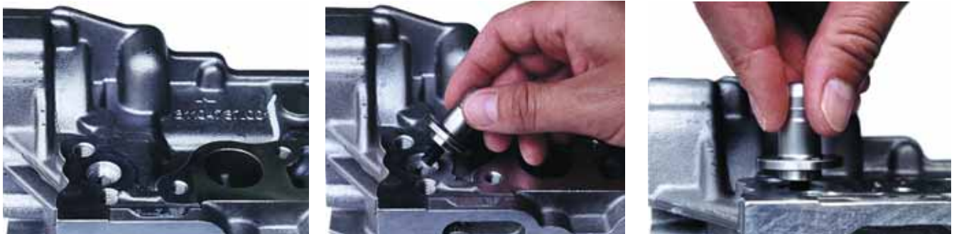
Mount retractable nipples (direct clamping of workpiece)
