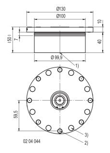
Hydraulic connection selection through floor or flange
