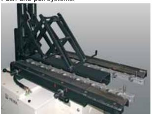
Pushing and pulling is carried out by means of a lever movement or using a centring tenon on the die cart.
