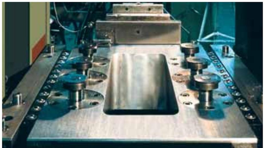
Pull clamping elements in the press bed of a double column press. Easy die positioning is ensured by roller blocs in the T-slots of the press bed.
