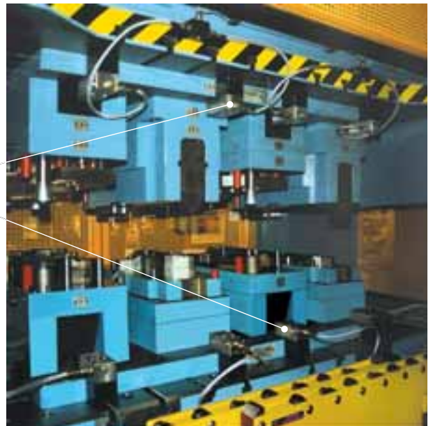
Sliding clamps fastened to bed and ram of a double column press. Dies are entered from the front using consoles.
