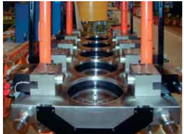
5-stage drop forging press equipped with wedge clamps with directional seat valves to activate the different stages
