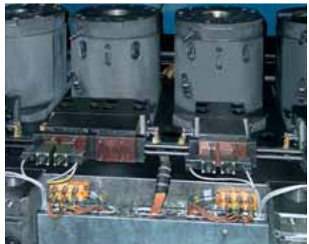
Wedge clamps with flanged directional seat valves. Clamping and unclamping positions are electrically controlled. Little installation work as a result of plug-type connections between the clamps.
