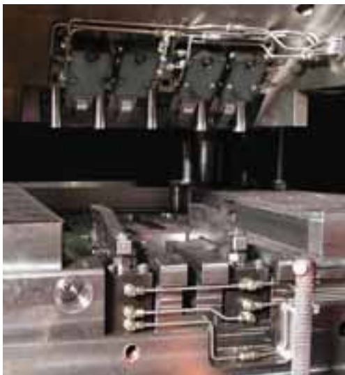
Use of wedge clamps with sequence valve control in a forging press
