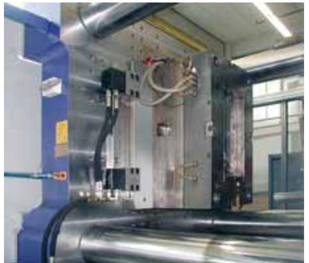
Wedge clamp with 160 kN clamping force on a Windsor W 550
