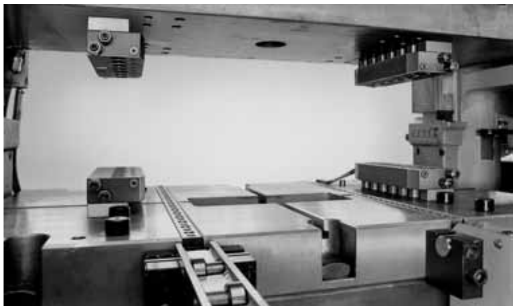
Clamping bars installed in press bed and ram. Easy loading of dies using die change consoles and lateral guide rollers.
