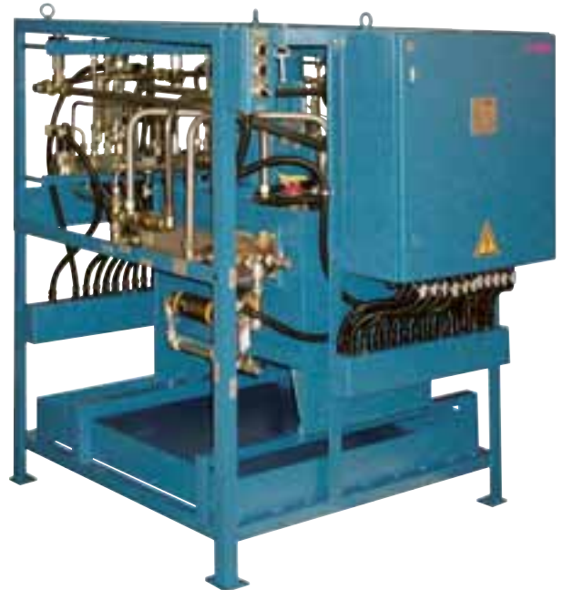
Frame-type unit for 3 forging presses: 12 clamping circuits with pressure reduction for compensation of temperature high-pressure 4.2 l/min., 400 bar cooling return 45 l/min., 10 bar
