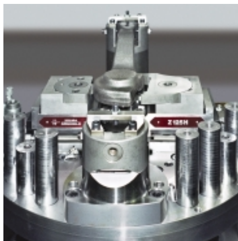
Self-centering vice hydraulically operated
