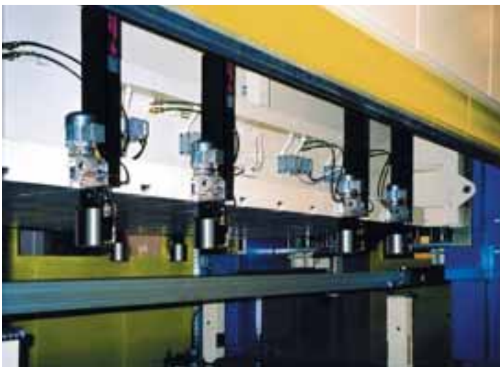
Use of rapid clamping systems with pusher chain on the press ram of a double-sided press
