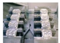
The clamping edge is milled off in the 2<sup>nd</sup> clamping step.
