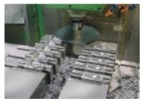
After finish-machining, the "lost head" is separated from the workpiece using a disk milling cutter.
