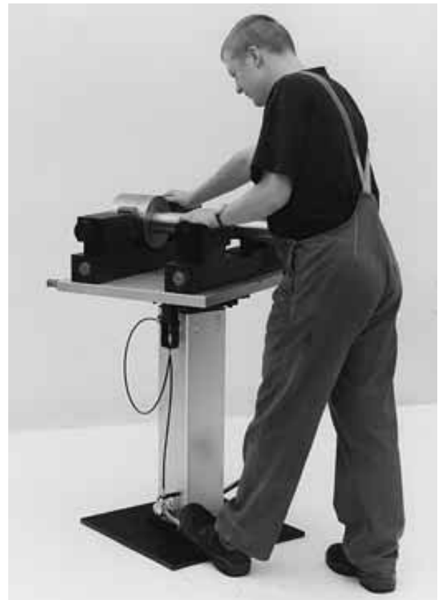
Concentric vice in preparation for machining of workpieces
