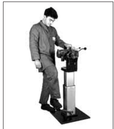
Swivel swivel element and extend lifting unit by foot operation
