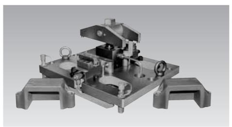
The clamping fixture in plate constructions installed on a vertical machining centre with rotary indexing table and trunnion bearing.
