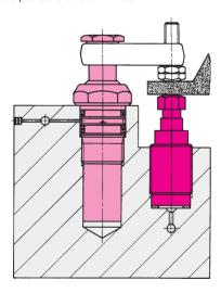
Support and clamping forces have to be adapted to each other, so that there will be sufficient force reserve available for the threaded-body work support to absorb the machining forces.
